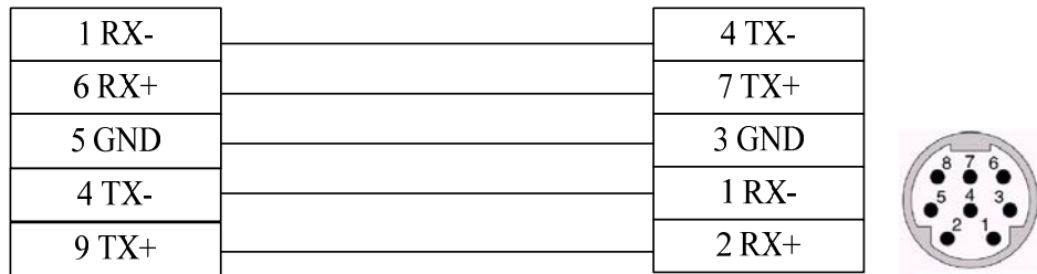
Pin assignment of 8-pin DIN round female connector
