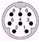
Pin assignment of 8-pin DIN round female connector
